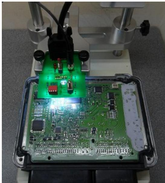
**3. Reading password: (This step is only necessary for TP8+).** Lift up the Boot DIP switches (D) as shown in the adapter overview on page 1, you can now read the password.
