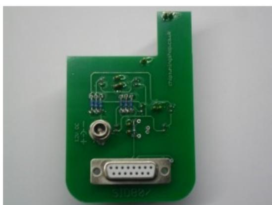
**1. Description:** This probe can be used for programming Continental SID807 TC1797 ECUs. It fits in most BDM positioning frames and is fitted with LEDs for accurate alignment on the ECU. Included with the probe is a 5mm perspex sheet.
