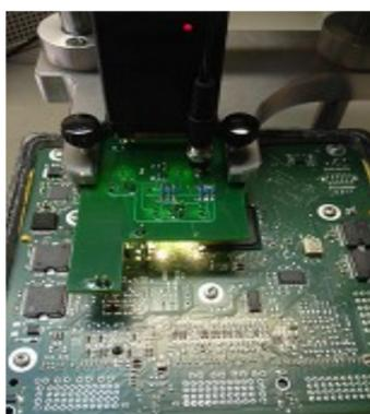
If lighting is required you can connect a 12V power supply to the jack on the probe (this only powers the LED's and not the ECU). It is possible to use the CMD power supply to power the LED's temporarily whilst aligning, once aligned you can return the power supply back into the CMD interface.
