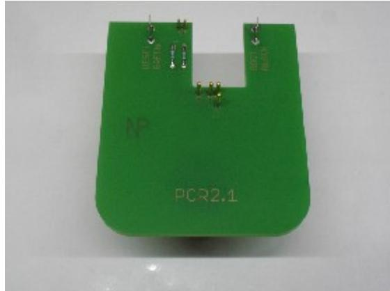
**1. Description:** This adaptor set can be used for unlocking and programming Simos Continental PCR2.1 ECU`s. It fits in most BDM positioning frames. Included in the kit is the PCR probe and an ECU adaptor cable set.
