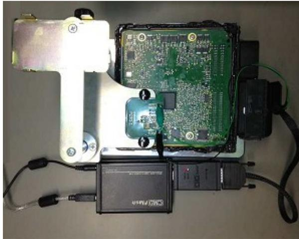
Adjust the ECU on the frame, then move the retainer carefully towards the ECU and ensure that all the pins are in their designated position. A diagram showing the location of the connections can be found on page 3.
